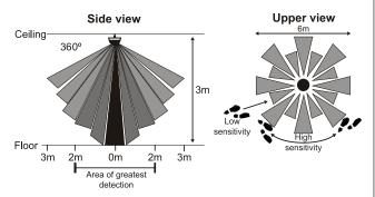
When the moviment is made against the luminaire, the sensitivity will be reduced.
